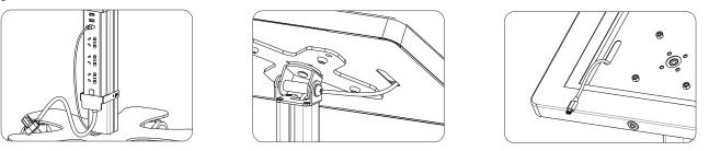
Assemble the lockable utility box (IPDMEUTBX, sold separately). Attach 2 brackets to the pole first, then fix the utility box onto the bracket securely.
