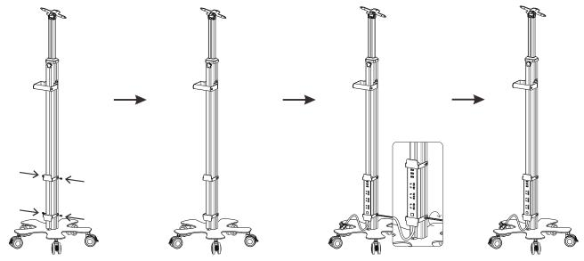
Wire your charging cable (not included) through the pole and connect to your tablet (not included) and power strip. See the suggested connecting method below:
